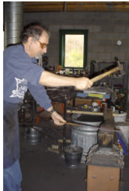
Photo 20: Do not be afraid of the the anvil. Step up close to it so you are not reaching for the work, but can strike downward with authority.
