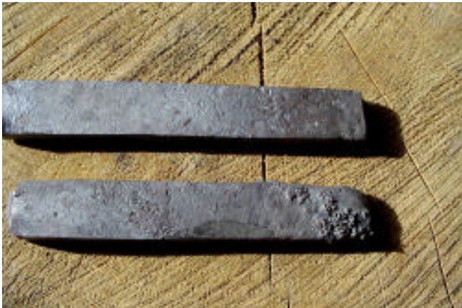
Photo 12: The bottom bar has been burned. The top bar has been burned then slightly up set and reworked— alas, the damage has been done.
