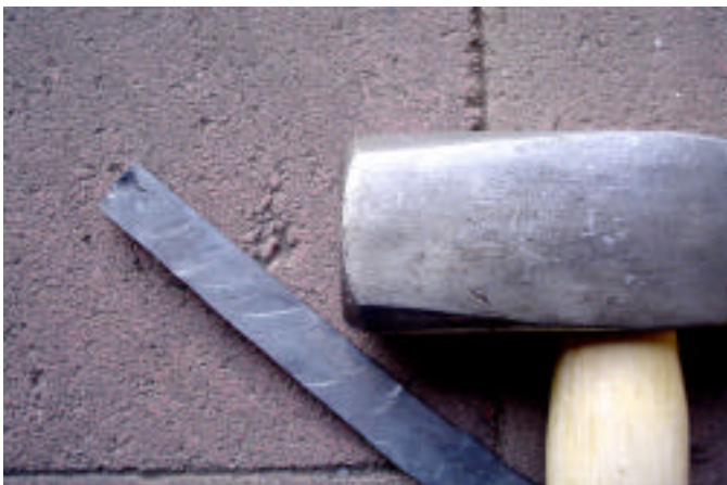
Photo 13: The marks left on the bar came from this poorly dressed hammer face.
