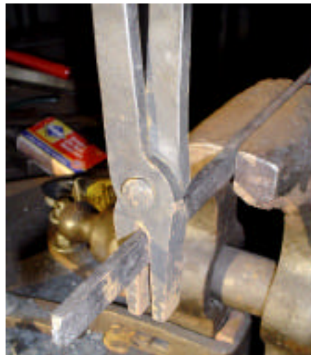
Photo 11: Correcting a twist with a pair of tongs and the bar held in the vise horizontally.
