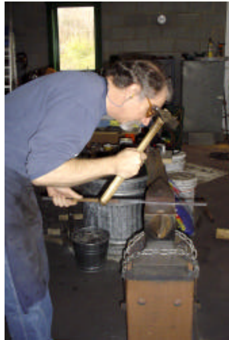
Photo 19: What is wrong with this picture? The bend at the waist is hard on the back. The face is more vulnerable to anything coming off the anvil. The waist bend also minimizes the travel of the hammer, hammer speed and the power of the blow are negatively effective. The grip close to the hammer head suggests the hammer may be too heavy. The "choked" grip shortens the arc of hammer travel. and the power of the blow.
