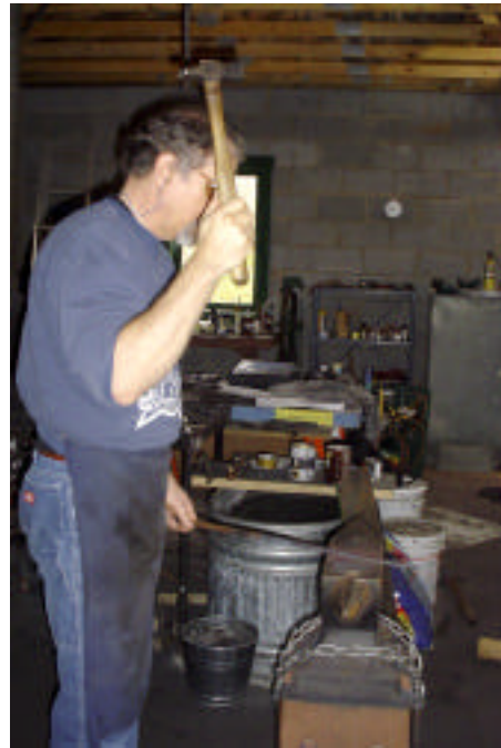
Photo 21: Perhaps not the paragon of forge technique, this smith is standing upright and is close to the anvil. He is gripping the handle near its end. He has raised his hammer out of his field of vision and is thus beginning to maximize the effect of the hammer swing.
