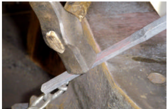
Photo 14: Scraping along a sharp anvil corner to get rid of scale before forging. Use the hammer head to apply downward pressure.
