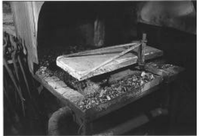
Forge set up for anthracite with swiveling refractory cover
