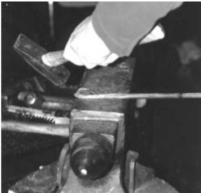
Flattening the outside face forges the center upwards
