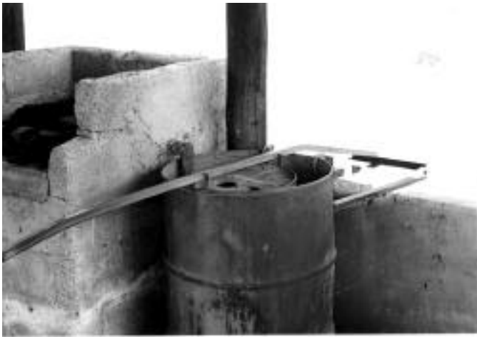
A drum bellows made from discarded materials
